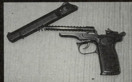
Slide is now released for removal.
