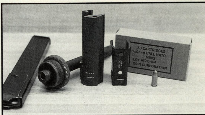
9mm conversion kit parts, from left: Sten magazine, 9mm barrel, bolt, and magazine adapter.
