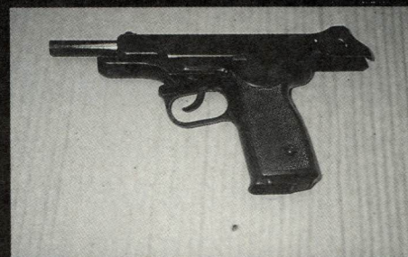
For disassembly: slide to the rear, pull trigger guard down.
